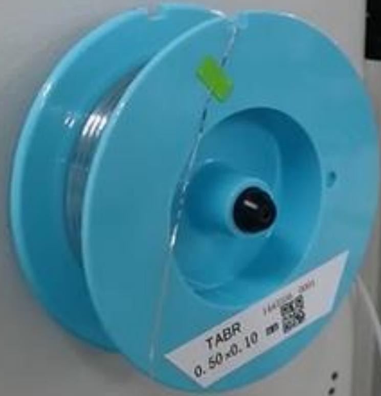
③ Hold the flange of the spool and remove it parallel to the shaft.
