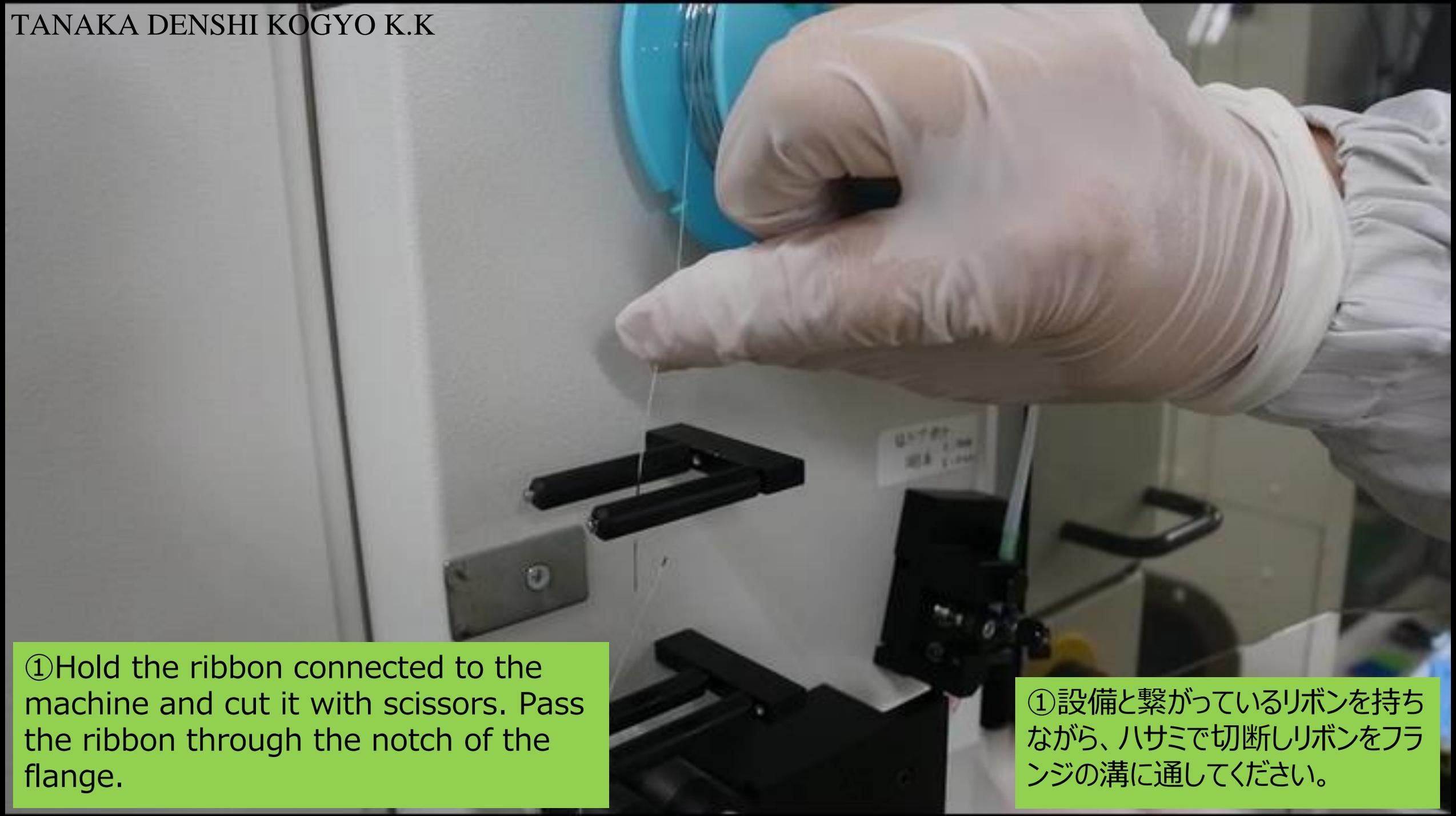
① Hold the ribbon connected to the machine and cut it with scissors. Pass the ribbon through the notch of the flange.
