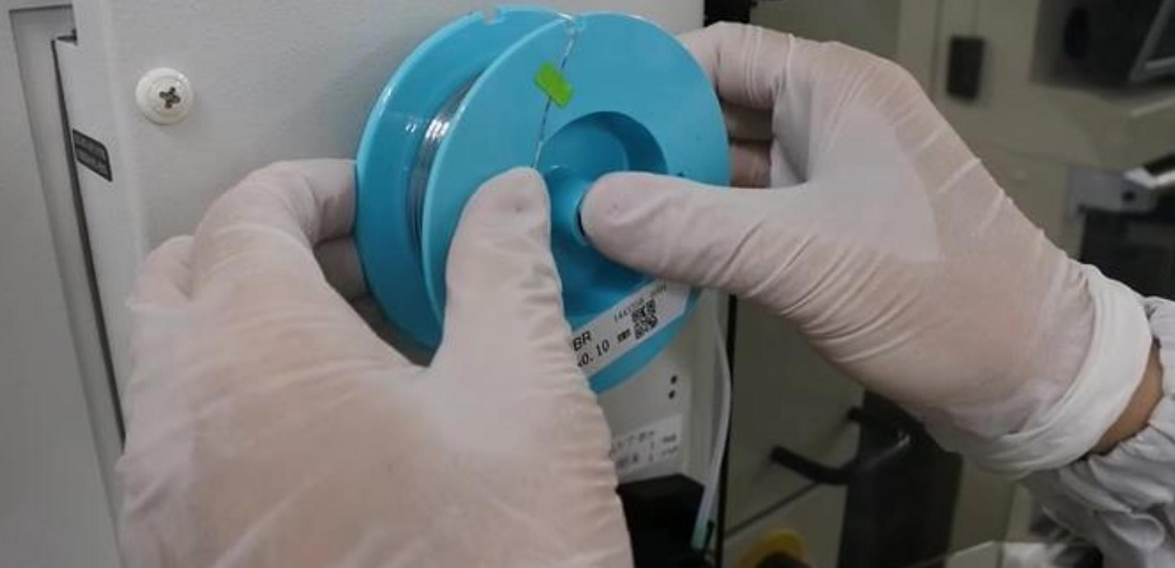
③ Hold the flange of the spool and remove it parallel to the shaft.
