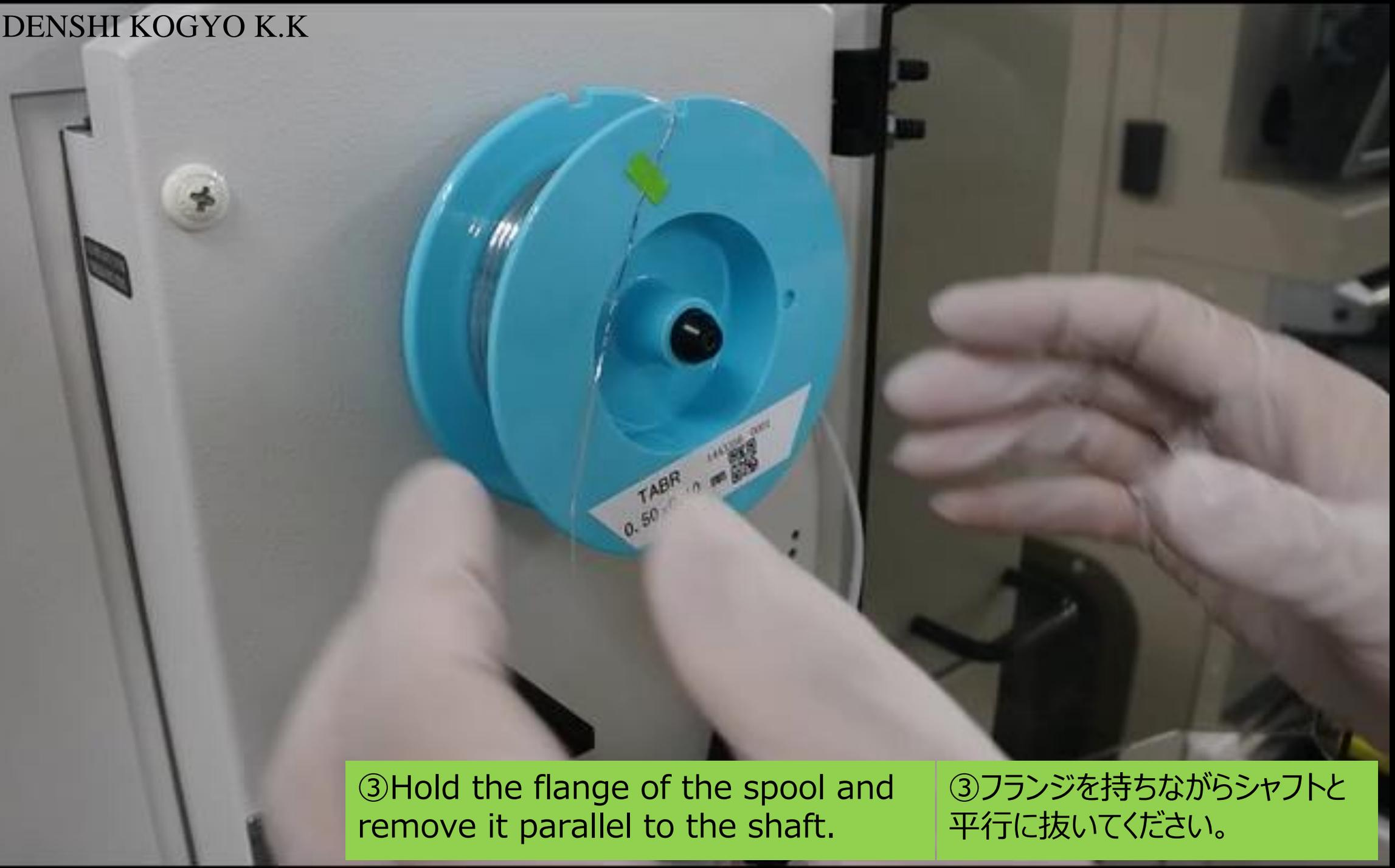
③ Hold the flange of the spool and remove it parallel to the shaft.
