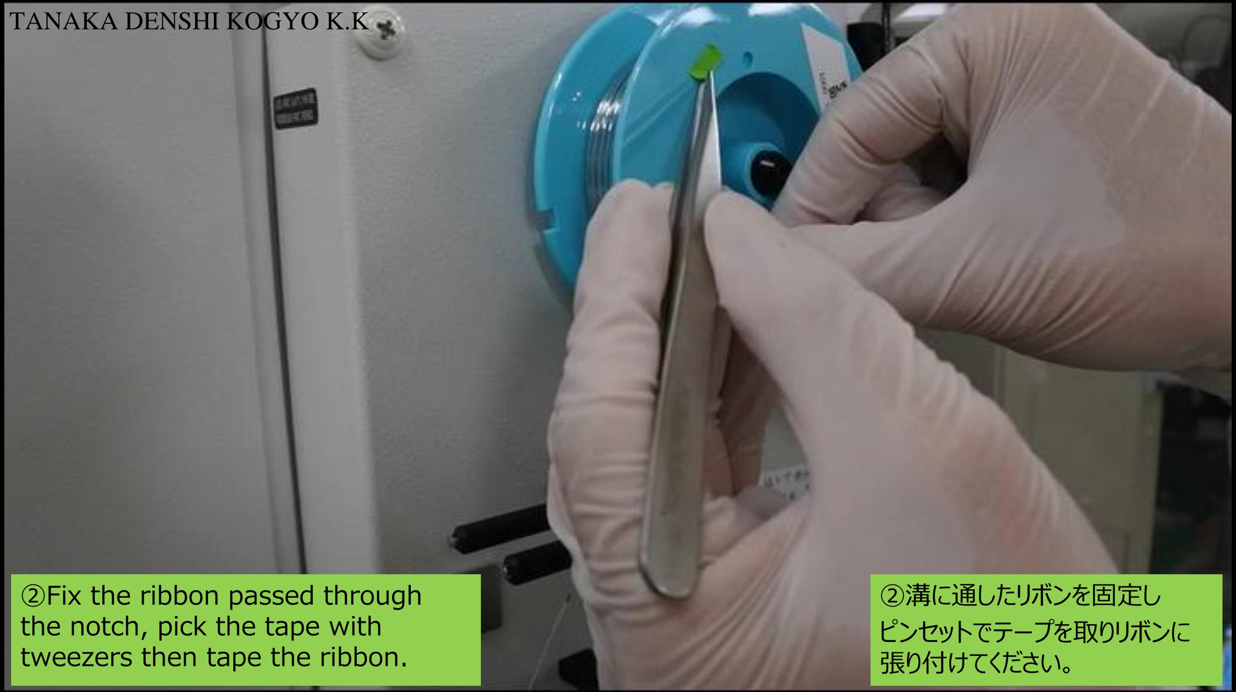
②Fix the ribbon passed through the notch, pick the tape with tweezers then tape the ribbon.
