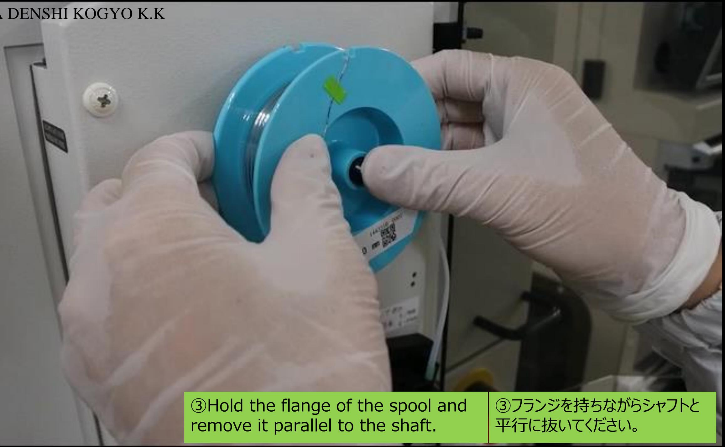
③ Hold the flange of the spool and remove it parallel to the shaft.
