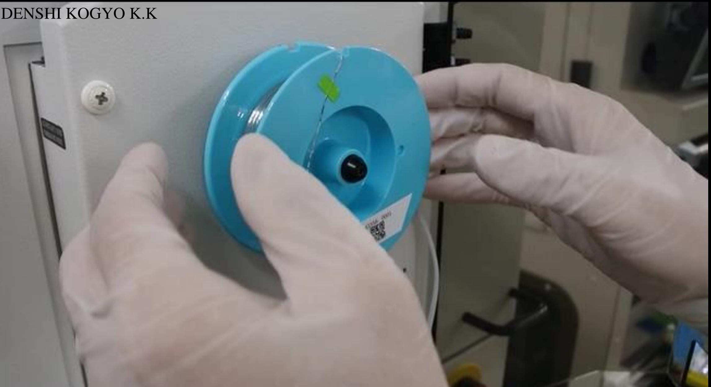
③ Hold the flange of the spool and remove it parallel to the shaft.
