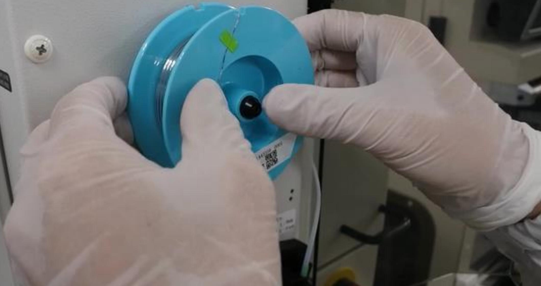
③ Hold the flange of the spool and remove it parallel to the shaft.
