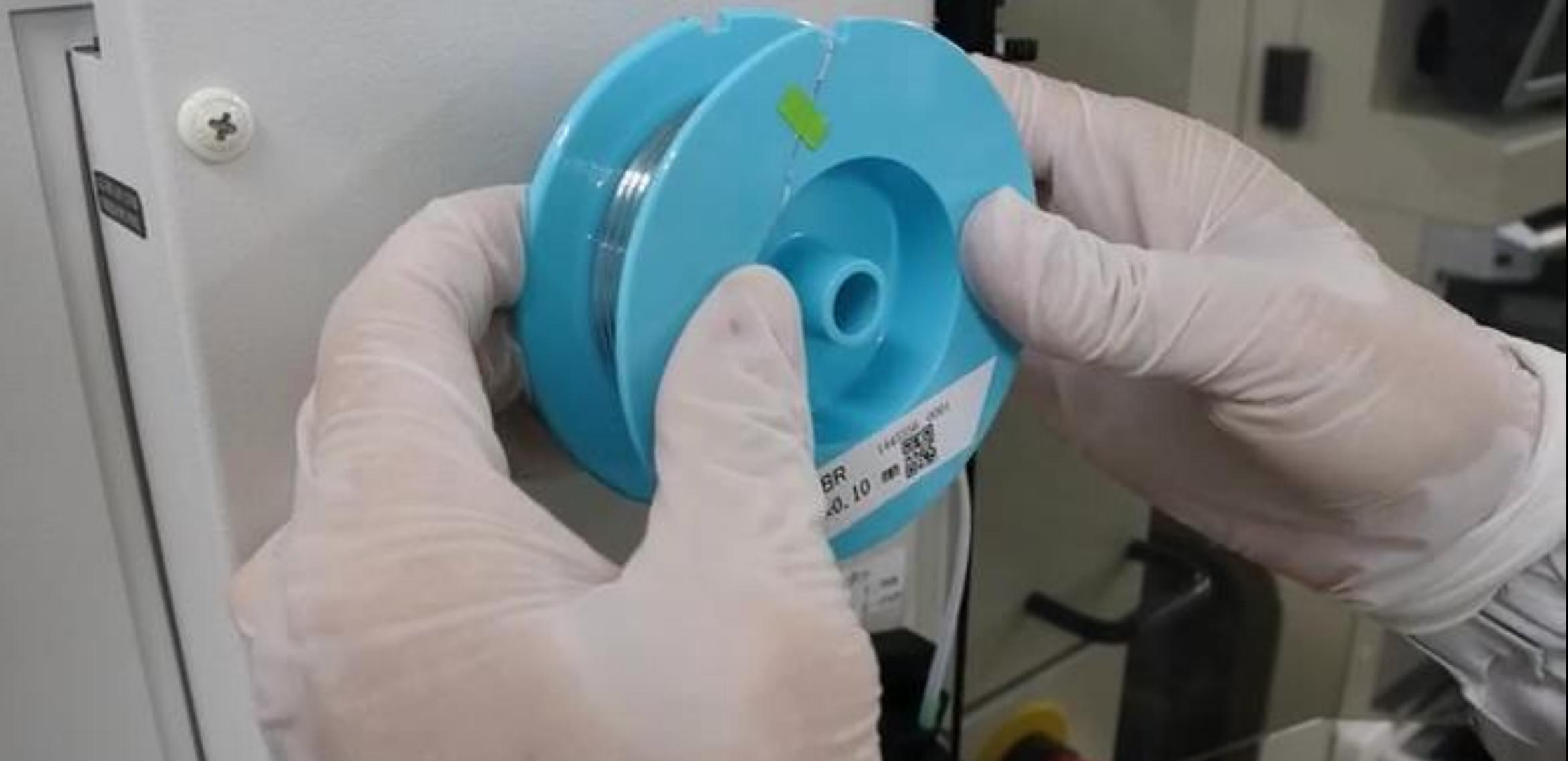
③ Hold the flange of the spool and remove it parallel to the shaft.
